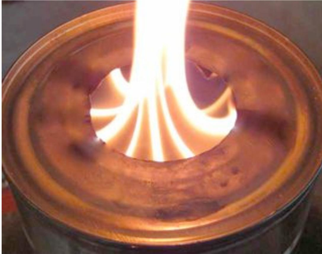
Seperate control of **Generation** and **combustion** of gas from biomass with very simple means.
