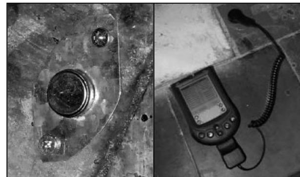
Temperature dataloggers as stove use monitors (Thermochron iButtons®)
