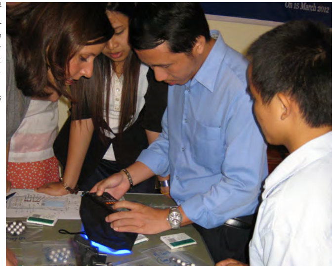
The FDA has developed a hand-held, battery-powered scanner that uses light wavelengths to highlight irregularities in antimalarial and other drugs.
